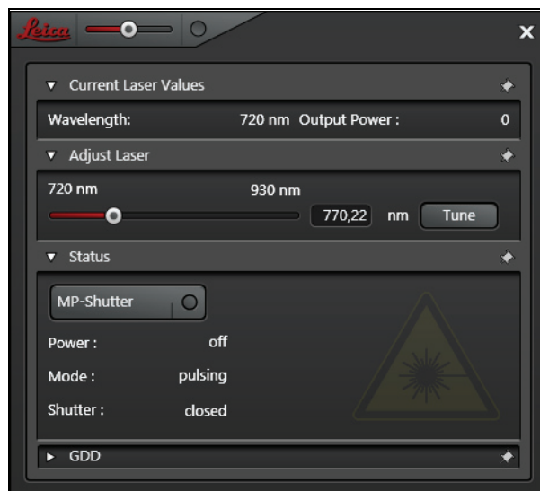
Figure 100: MP Laser Configuration, second shutter closed
