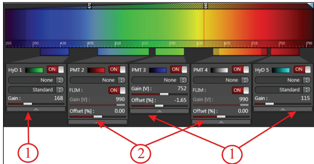
Figure 114: Beam Path Settings of LAS AF when using detectors for default image acquisition (1) and internal FLIM detectors for intensity image acquisition (2)
